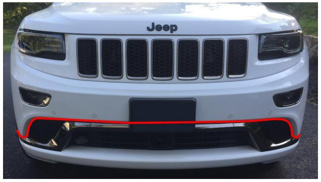
6) Once the clips are out, work your hand around the lower fascia pulling gently starting from the outside corners and working in. A second set of hands may be necessary to support the fascia and prevent it from falling to the ground.
